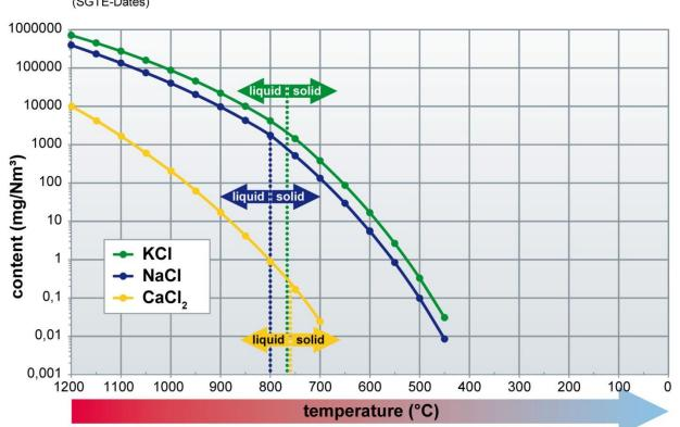
Typical content of a gaseous salt after firing zone in WTE and biomass plants in the range below 1000 mg/Nm3
