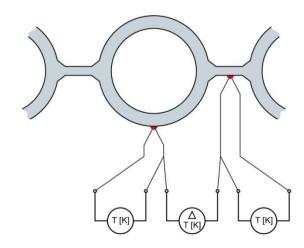
Two thermocouples are one sensor (one at fin position and one at crown of tube)
