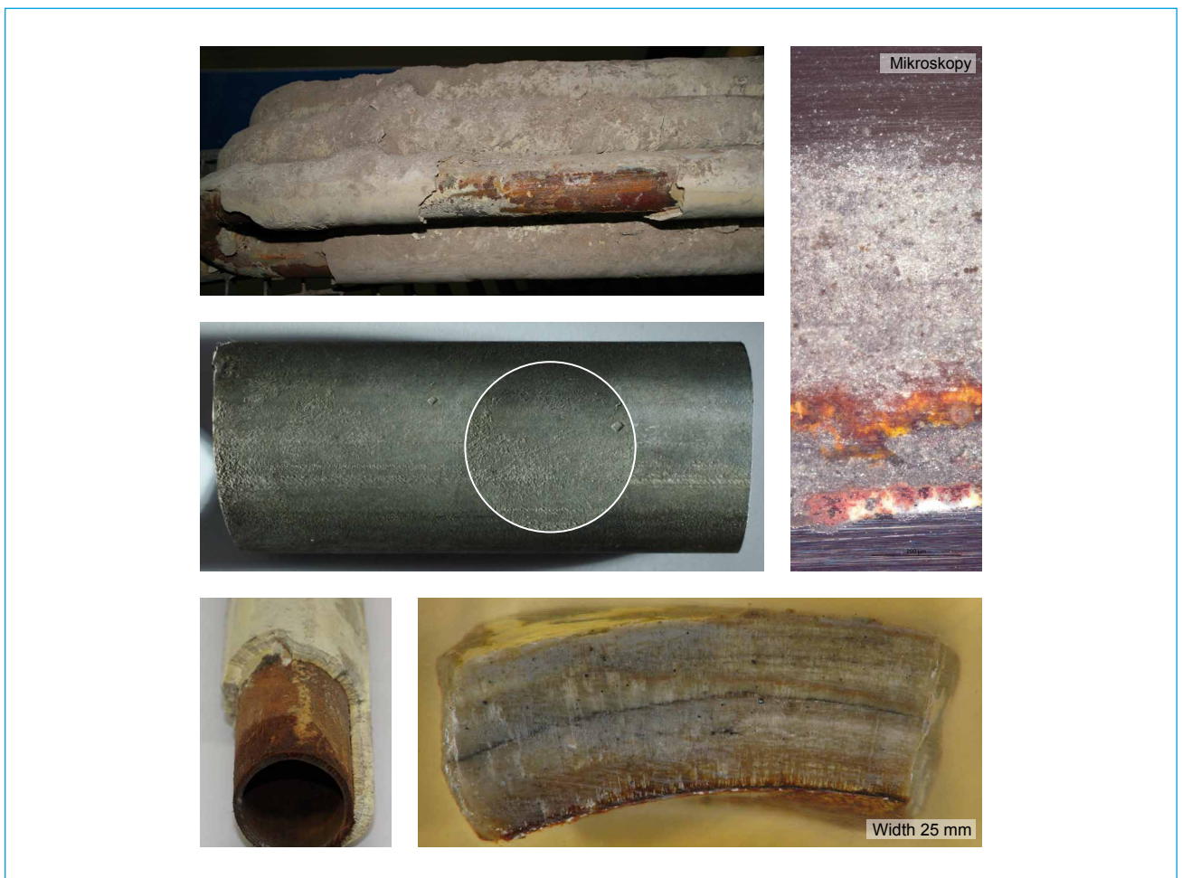
Figure 7: Provocation test at a WTE plant at a medium temperature of 90°C, flue gas temperature of about 235°, after around 4,000 operating hours, under the influence of SNCR.
