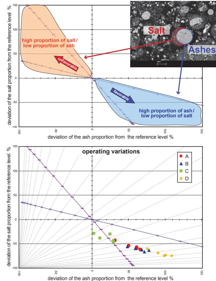
Taking the chemical composition of each sample the position in the ASP diagram can be calculated.
